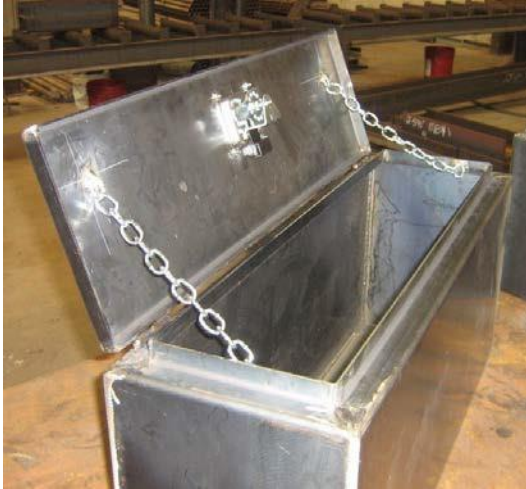
Toolbox Manufactured from quality 10-gage A36 material
